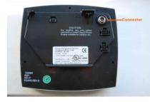
All valves are low voltage valves with a 240V transformer. With the power off connect the transformer provided to 240V supply. With the power OFF plug the flying lead into the connecter on the controller (Fig A.11). If you have an in line transformer this needs to be wired into a fused switch. Ensure that the flying lead cannot get caught on the camshaft or any of the valves moving parts. Fig A.11
